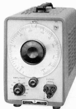
Fig. 2. (right) New -hp- Model 207A oscillator covers complete 20 cps-20 kc range in single band, has shaft extension at rear to enable it to be used with external motor drives for automatic audio response measurements on amplifiers, transformers, speakers, and other audio devices. No zero setting is required. Log dial facilitates response plots on scope or recorder.
